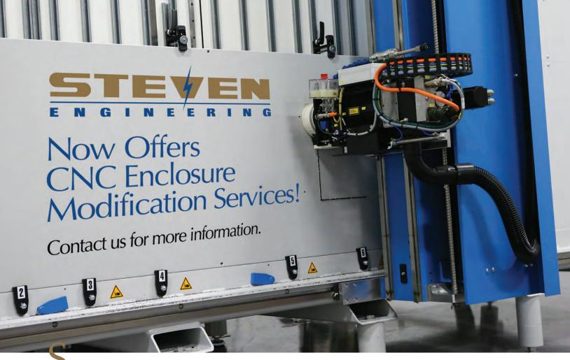
teven Engineering now has the capability to custom configure enclosures to meet all of your requirements. By using the state-of-the art Steinhauer eCAB ModCenter, we are able to offer an almost endless variety of options to fulfill the most demanding specifications. We have the capability to machine fiberglass, polycarbonate, sheet steel, copper and even stainless steel!
