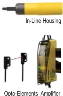
3. **Fiber optic systems:** Sensing systems in which fiber optic cables are used with either remote or self-contained sensors. Fiber optic devices have no electrical circuitry and no moving parts, and can be used to safely pipe light into and out of hostile environments.
