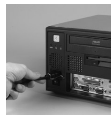
Plug ring-lock securely fastens the power cord
