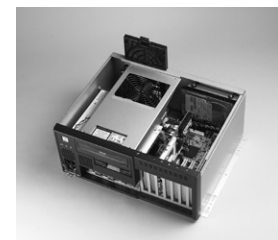
Solid disk drive housing & easy-to-maintain fan filter
