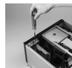
User-friendly mechanical design for installing an add-on card
