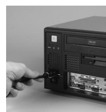
Plug ring-lock securely fastens the power cord
