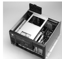
Solid disk drive housing & easy-to-maintain fan filter
