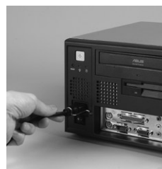
Plug ring-lock securely fastens the power cord
