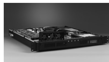
Three filtered 10-CFM cooling fans at the front
