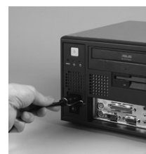
Plug ring-lock securely fastens the power cord
