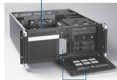
Reusable and easy-to-maintain fan filters
