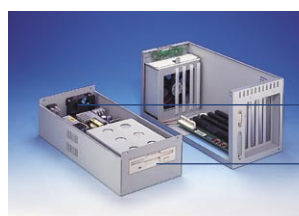
One 14-CFM cooling fan One 3.5" drive bay
