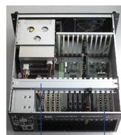
Hold-down clamp Max. 14-slot backplane
