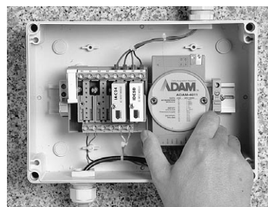
DIN-rail installation No screws; just snap the module in place. Offers space for three modules.
