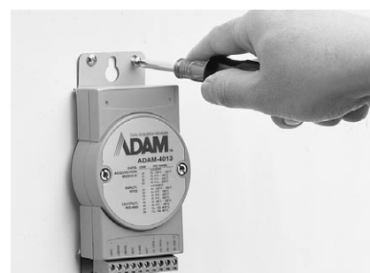
Panel/Wall Mounting Use this special bracket to mount modules on any flat surface
