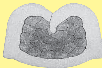
B shape cross section stamped contact
