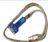
Serial USB Cable for Modem Download CA6-USB232-01
