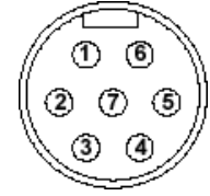
Face view of the receiver receptacle (1" – 16UN – 2A thread)
