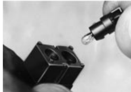
1. Insert solder terminal receptacle into hole in base of panel mount unit.
