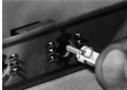
1. Insert the PWB receptacle/incandescent lamp assembly through a hole in the printed wiring board.
