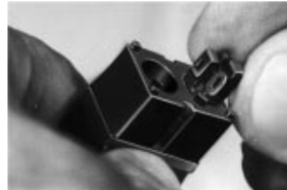
2. A 1/8-turn clockwise applied to the receptacle locks it in the base.
