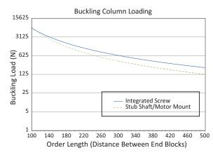
Note: Based on 500 mm stroke, GST version with .125 C.O.F. and .3G acceleration. Based on 24 volt, but higher voltage amplifiers may produce higher speeds.
