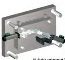
All-electric replacement for hydraulic cylinders improves throughput with servo control and lower maintenance for corepull cylinders. A typical 3 inch stroke GSM Series actuator used in a valve-modulating application can control position to +/-0.5% and fully open or close in less than 200 mSec.
