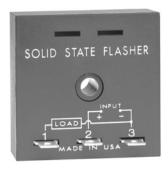
The FS200 Series may be used to control inductive, incandescent, or resistive loads. Input voltages of 12, 24, 36, 48, or 110VDC are available. Factory fixed flash rate of 90 FPM or may be ordered with a fixed custom flash rate ranging from 10 to 180 FPM. Encapsulation provides protection against shock, vibration, and humidity. Uniform performance, high inrush current capability, and low RFI, make this series ideal for general industrial applications.
