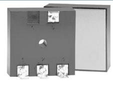
The AF Series offers a high inrush capacity of up to 200A. These devices exceed mechanical type relays in both performance and lifespan. The AF Series is constructed with no moving parts to arc, wear, and eventually fail; 100 million operations are typical. Circuitry is encapsulated to provide protection against vibration and moisture, making the AF Series ideal for outdoor applications.
