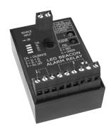
The FB series is a universal lamp alarm relay designed to sense the failure of flashing LED beacon lamps. It will monitor the operation of one to eight beacons connected to a single flasher and/or auxiliary modules and the operation of the flasher. The FB Series output relay energizes when one or more lamps fail. All monitored lamps must be the same wattage and voltage. The 0.5A solid-state output energizes when a flasher failure
