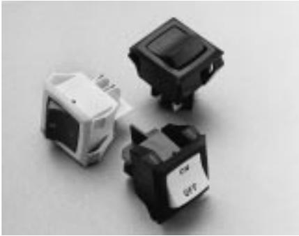
The RGSC-Series Super Corvette rocker switches offer the Corvette styling in a double pole construction with higher electrical ratings and high inrush capabilities. These switches can handle up to 125 amp peak inrush current and can accommodate a wide range of panel cutouts due to the patented mounting ear construction. International ratings are available up to 20 amps.
