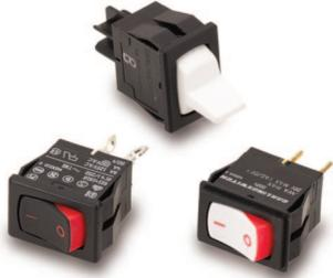
The patriarch of the Carling line of sub-miniature switches has its roots deep in the Appliance, Audio Visual, Power Supply, and Telecom markets. The 611/621-Series compact size, sleek styling, actuator and termination choices make this switch a cost effective solution to most any switching need. International approvals, single or double pole circuitry, and ratings to 11A 125VAC further the broad appeal of this product family.
