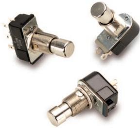
The 110-Series provides a compact yet rugged solution to general purpose switch needs. Alternate action, metal construction and stiff (6-8lb.) actuation force have combined to make this switch a pillar in the Music Industry and Audiovisual Markets. This versatile switch is available in maintained and momentary circuits with a variety of termination options.
