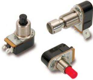
The P26-Series pushbutton switches are single pole, AC rated for 8 amps at 125 VAC and suitable for shallow back panel applications. These switches are momentary action with a medium actuation force (13 oz. typical). The P26-Series switch is equipped with a slow-make, slow-break contact mechanism. Typical applications include usage for an Alarm or Warning Device, as well as Test and Measurement Equipment.
