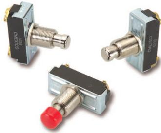
The 170/172-Series pushbutton switches are single pole, high amperage switches suitable for shallow back panel applications. These switches are momentary action and require an actuation force of 2.5 lbs. The 170/172-Series switches are equipped with a slow-make, slow-break contact mechanism and are rated at 15 amps at 125VAC.
