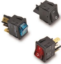
A high powered offering packed into a compact sized envelope, the 622/632-Series is a staple of the Appliance, Food Service, Transportation, and General Purpose markets. The silver-alloy butt contacts will handle inrush spikes up to 125 amps and steady state current to 16A 125VAC. The lighted 632-Series features a multitude of illumination circuit options available with LED, incandescent and neon style lamps.
