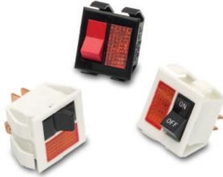
The TLG-Series Mini Tippette snap-in rocker switches are single pole, rocker or paddle actuated with an adjacent indicator light. These single-actuator-switches are AC rated to 20 amps and are also suitable for low voltage DC applications, in a wide range of markets including Appliance, HVAC, Food service and Transportation.
