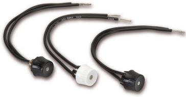
The R135 and R135A-Series rotary switches are single pole, single throw “L” rated up to 3A, feature an ON-OFF repeating action, and are available with a nylon actuating knob; nylon snap-in bracket or nickel-plated brass bushing. These switches are typically used to control lighting functions.
