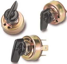
The 700 and 800-Series are single pole multi-position, general purpose rotary switches. These switches feature a nylon actuator in a metal clad construction along with a self-cleaning silver plated contact design. The 700 and 800-Series are typically used in applications requiring multi-position speed controls, such as electric fans.
