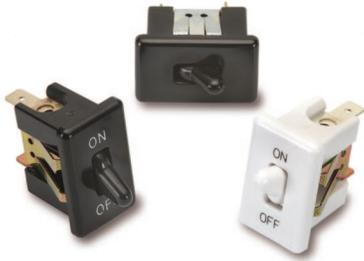
The MAAOA/215-Series toggle switches are single pole, AC rated at 20 amps and 125 VAC. These switches are snap-in mounted, with a phenolic toggle and base, and are suitable for high ambient temperature applications including Coffee Makers and Food Warmers.
