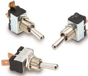
The C-Series single pole compact high current toggle switches are ideal for applications with back panel size constraints. These switches feature self-cleaning contacts and ratings up to 20A 125VAC, 10A 250VAC, 1 1/2 HP 125-250VAC. With a rugged metal construction, these switches figure prominently in the Environmental Controls, Marine, Food Service, Vacuum Cleaner and various other general purpose markets with stringent current carrying requirements.
