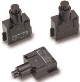
The new PP-Series plastic pushbutton switches are heavy-duty, single pole switches with wire leads. They are alternate action, available in single throw construction, with AC ratings up to 15 amps. Both bushing and bracket are made out of nylon. These high current switches are popular with in the Appliance market.
