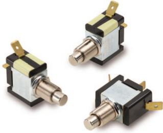
These rugged pushbutton-type switches feature international approvals, ratings to 20A 125VAC and a heavy actuation force (3-5 lbs. typical) which makes this switch ideal for use as a “foot-pedal” switch. These switches have become mainstays for canister Vacuum Cleaner applications. The metal bushing and plunger construction enables this alternate action switch to withstand the rigors of most any stringent pushbutton application.
