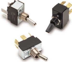
General purpose workhorses with options tailored to meet most any need. Ratings to 20A 277VAC, international approvals, various actuator, bushing, termination, and circuit choices allow this toggle switch to easily integrate into a variety of different applications. The G-Series has a storied history in the Marine, Food Service, Generator, Industrial Control, and Office Automation markets and is appropriate for usage in low voltage DC applications as well.
