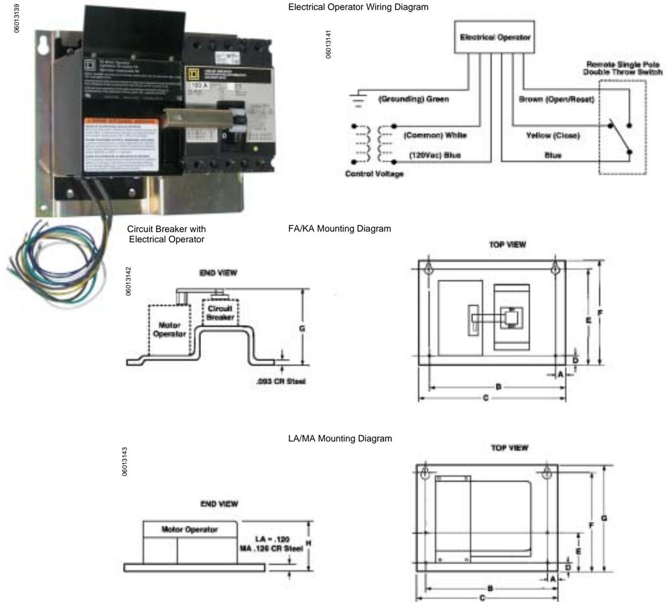
Table 65: Electrical Operator Mounting Dimensions, Inches (mm)
