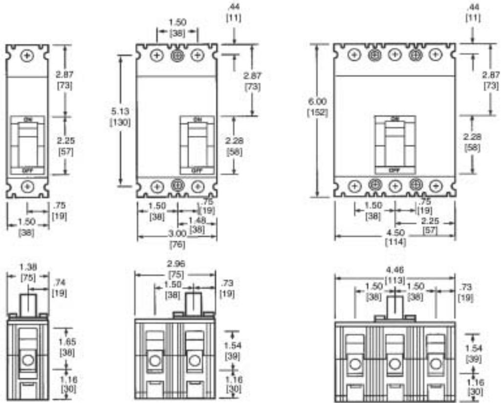
FCL 2-pole circuit breaker dimension is the same as a 3-pole circuit breaker.
