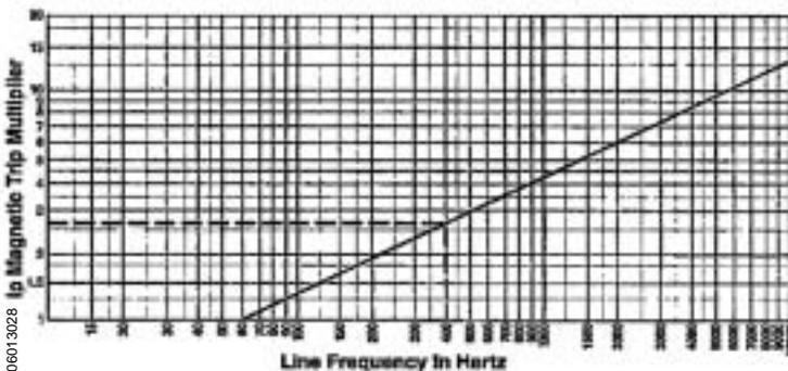
At frequencies above 60 Hz, more current is necessary to magnetically trip a circuit breaker than at 60 Hz. The figure below shows the multipliers of 60 Hz current that it takes to magnetically trip a circuit breaker when applied at various frequencies. For example, at 60 Hz it takes 1000 amperes to magnetically trip a 200 ampere KA circuit breaker at its low setting. At 400 Hz it takes 2600 amperes (2.6 multiplier) to magnetically trip the same circuit breaker.
