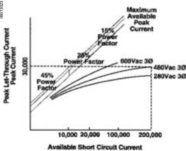
Let-through current curves show the extent to which a current limiting circuit breaker limits the peak current that could flow during a short circuit. On these curves, the slanting straight lines marked 15%, 25% and 45% power factor show the maximum theoretical peak currents that could flow in a faulted circuit having that particular short circuit power factory—with NO current limiting device in the circuit.
