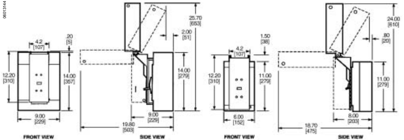
Mounting Dimensions for Electrical Operator Mounted on MAL or MHL Circuit Breaker or Switch
