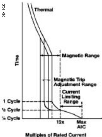
The right hand portion of a tripping curve displays the magnetic tripping response of the circuit breaker. This takes place when overcurrents of sufficient magnitude operate an internal magnetic armature that unlatches the tripping mechanism. Magnetic tripping occurs with no intentional delay.
