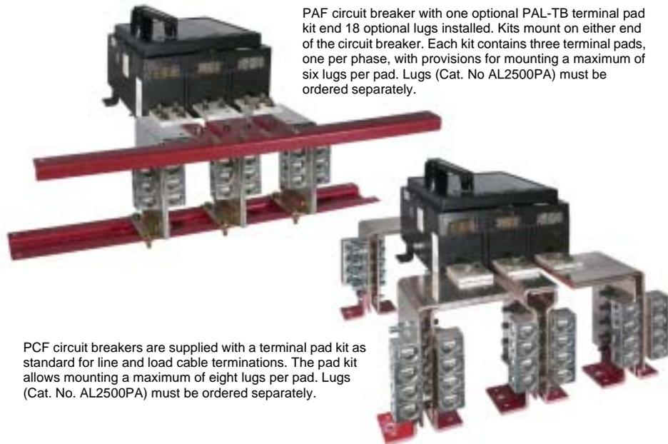
PAF circuit breaker with one optional PAL-TB terminal pad kit and 18 optional lugs installed. Kits mount on either end of the circuit breaker. Each kit contains three terminal pads, one per phase, with provisions for mounting a maximum of six lugs per pad. Lugs (Cat. No. AL2500PA) must be ordered separately.
