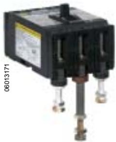
Rear connecting studs are designed to allow rear termination in applications, such as control panels where wire gutter space may be limited. The studs can be bolted directly to the bus bars or lugs can be attached to the studs. Long and short studs should be alternated on adjacent poles to assure proper electrical clearance. These studs are not UL Listed.
