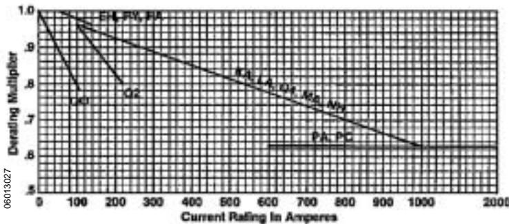
At frequencies above 60 Hz, the interrupting capacity of thermal-magnetic circuit breakers is less than the 60 Hz interrupting capacity. Unless specifically marked on 400 Hz systems, the interrupting capacity of Square D® circuit breakers is reduced to 1/10th of the 60 Hz interrupting capacity.
