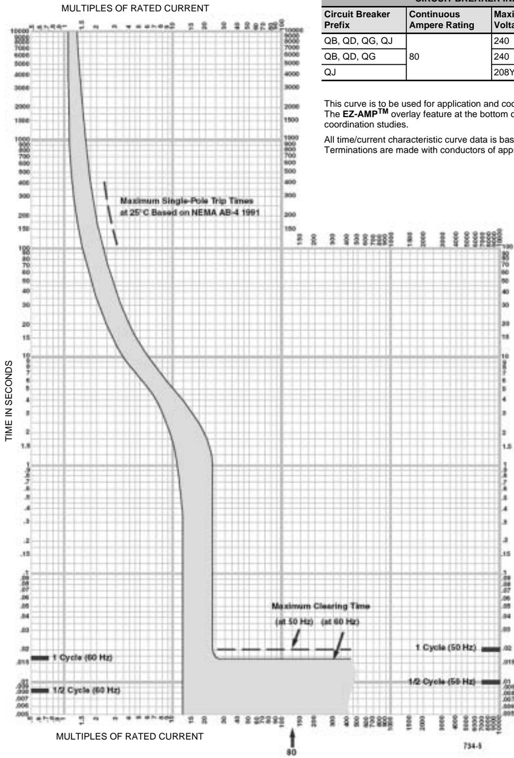
This curve is to be used for application and coordination purposes only. The EZ-AMP™ overlay feature at the bottom of the page should be used during coordination studies. All time/current characteristic curve data is based on 40°C ambient cold start. Terminations are made with conductors of appropriate length and ratings.
