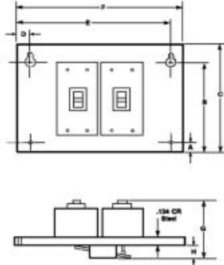
Requires two circuit breakers with WB suffix, one walking beam assembly and one mounting pan.
