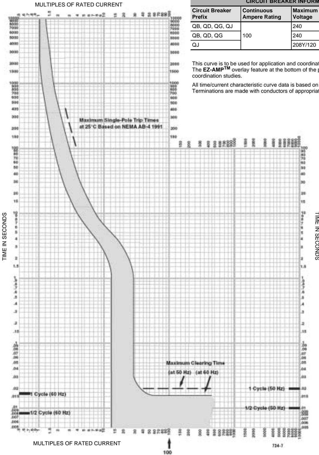
This curve is to be used for application and coordination purposes only. The EZ-AMP™ overlay feature at the bottom of the page should be used during coordination studies.
