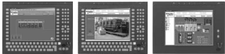
Screens for Modular iPC industrial PCs (any screen can be used with any type of Control box)
