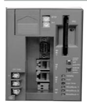
Communication 2 Modbus ports, 1 Modbus Plus port, 1 PCMCIA II slot interfaces Conformal coating No Yes No Yes Railroad standard EN 50155 No 96 K words **Total data memory** 48 K words Memory Startup RAM RAM 32K 512K 64K 1 Mb Flash PROM PCMCIA II card 1 Mb 1 Mb Logic memory for Modsoft LL 32K words 620 kB 16K words for Concept IEC
