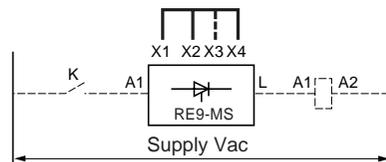
Link to be made between terminals X2 and X4 on one side and X1 and X2 on the other side.
