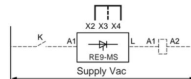
Link to be made between terminals X2 and X4.
