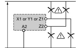
⚠ No galvanic insulation between supply terminals A1, A2, B1, B2 and control inputs X1, Y1, Z1, Z2.
