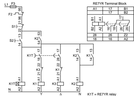
⚠ No galvanic insulation between supply terminals A1, A2, B1, B2 and control input Z2. This terminal must therefore never be used (factory setting).
