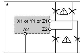
⚠ No galvanic insulation between supply terminals A1, A2, B1, B2 and control inputs X1, Y1, Z1, Z2.
