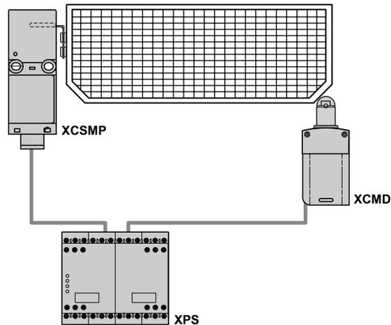
Locking by operating key and actuation in positive mode with a safety relay
