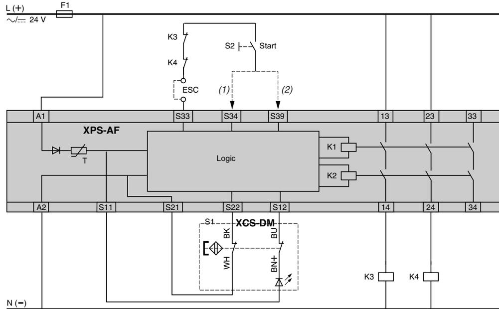
(1) With monitoring of start button. (2) Without monitoring of start button. ESC: External start conditions.
