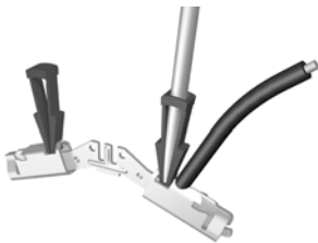
Principle of insulation displacement technology
