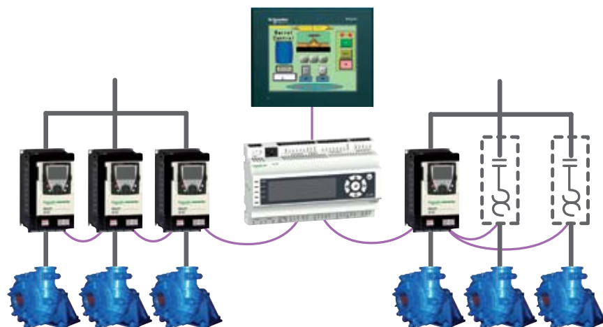
Multiple-pump system connected to a single intelligent controller and HMI
