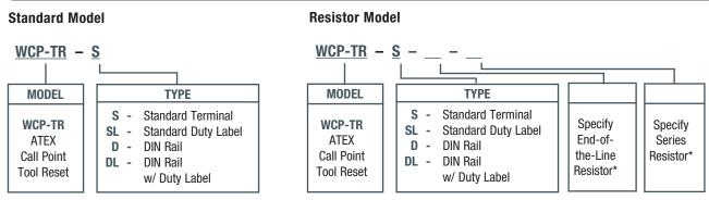
\*End-of-line and/or series resistor that must be included at time of order. 259366A Rev A
