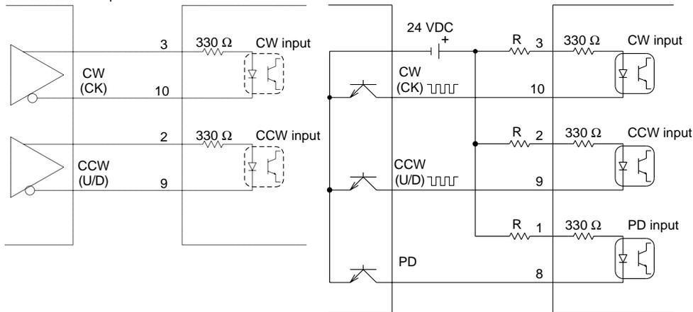
For a signal power supply of 24 VDC, connect an external resistor R (1.3 kΩ 1/2 W) in order to hold the current to 15 mA or lower.
