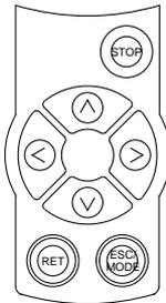
As shown above, 6 modes are available. (I/O mode and MON mode do not function with this driver.) When the communication mode is started by the teaching box, a menu can be selected with [ESC/MODE]. Select the mode indication LED for the mode to be implemented (all mode indication LEDs turn Off in the ID mode) and press [RET] to start each mode. Refer to the instruction manual for the operation of each mode.
