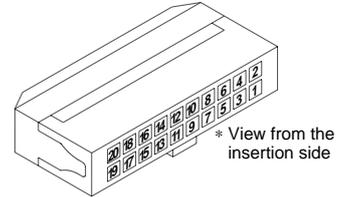
A ▽ mark is located on the connector number 1 side.
