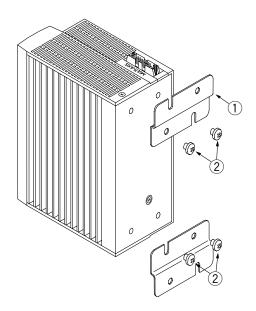
Perform by mounting the attached bracket. For mounting dimensions please refer to the external dimension on the prior page. For wall mounting, please prepare the required M5 screws (4 pcs.).
