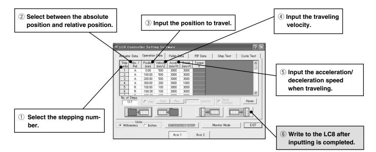
Able to input the stepping data by using controller setting software.
