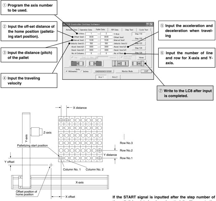
If the START signal is inputted after the step number of the palletizing data has been inputted, it will move to the 1st row/1st column of the pallet.
