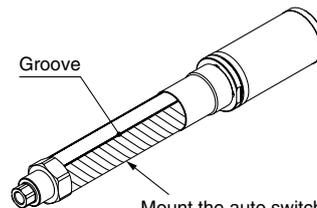
Mount the auto switch within the installation range (shadow portion). Otherwise, the auto switch may not activate.
