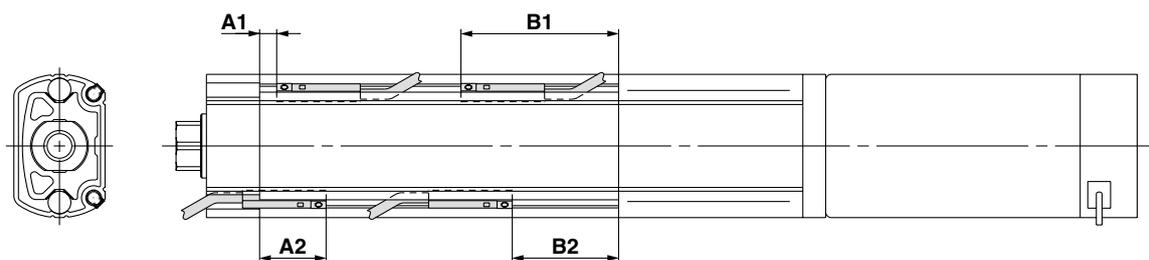
Auto Switch Mounting Position for Stroke End Detection
