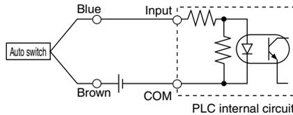
Connect according to the applicable PLC input specifications, as the connection method will vary depending on the PLC input specifications.
