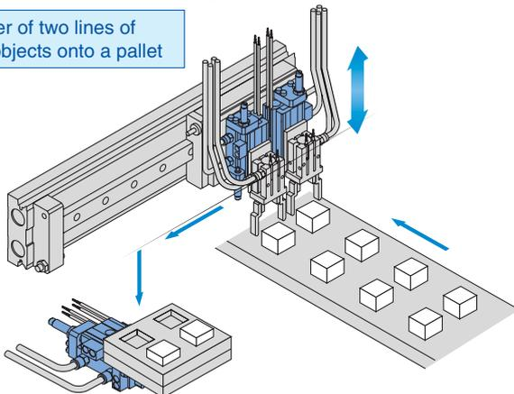
Sorting of work pieces of different shapes continuously supplied by a conveyor, etc.
