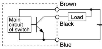
(Power supply for switch and load are separate.)
