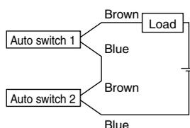
When two auto switches are connected in series, a load may malfunction because the load voltage will decline when in the ON state.
