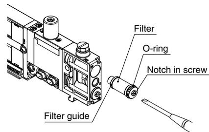
After tightening the plug (M-5P) with a tightening torque of 1 N·m, or manually tightening, use the tightening tool and tighten it by 1/4 turn.
