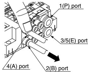
Hold down part of the release bush with your finger or a similar tool, as shown in the diagram, and pull out in the direction indicated by the arrow.
