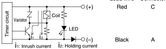
For the VQD1151W specifications (energy saving type), power consumption at holding is reduced with the above circuit. Refer to electrical power waveform as shown below.
