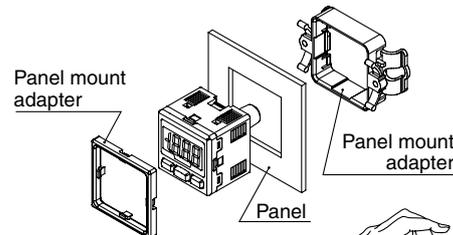
To release push the clips outward as shown on the picture, and pull back towards you.
