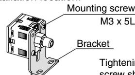
Tightening torque for bracket mounting screw should be 0.5 to 0.7 N·m.
