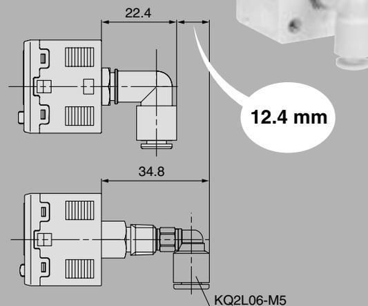
\* Comparison when One-touch fittings (KQ2H06-M5 / KQ2L06-M5) are connected to the piping ports (M5 x 0.8)
