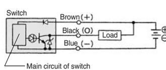
**Connection with PLC at negative COM terminal**
