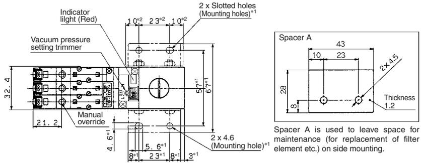
Spacer A is used to leave space for maintenance (for replacement of filter element etc.) on side mounting.
