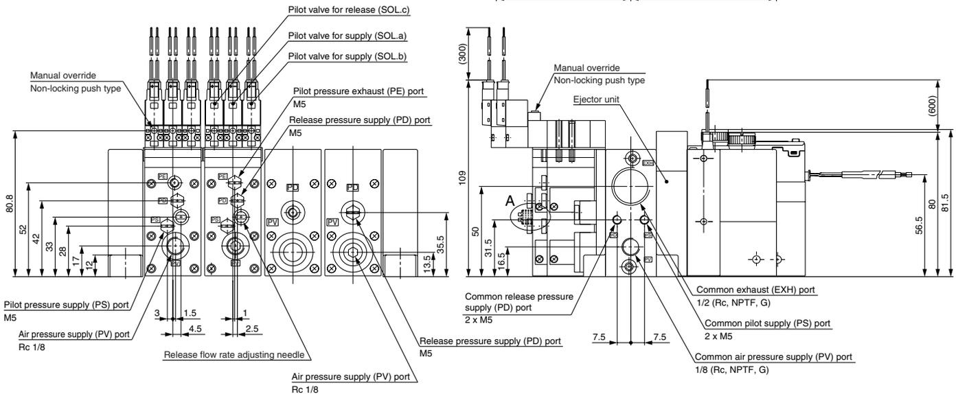
\* 1 The common exhaust port (EXH.) is also used as the pilot pressure exhaust (PE) port of the pilot valve. Use while the port is open to the atmosphere.
