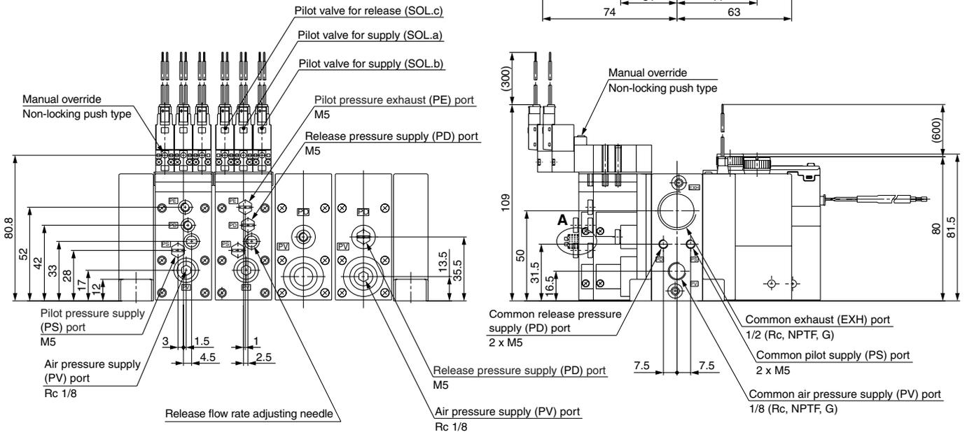
\* 1 The common exhaust port (EXH.) is also used as the pilot pressure exhaust (PE) port of the pilot valve. Use while the port is open to the atmosphere.
