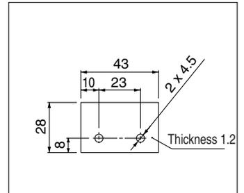
Spacer A is used to leave space for maintenance (for replacement of filter element etc.) on side mounting.
