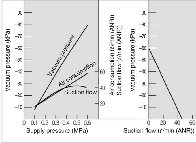
**ZR1-W18L1 Exhaust characteristics** **Flow characteristics**
