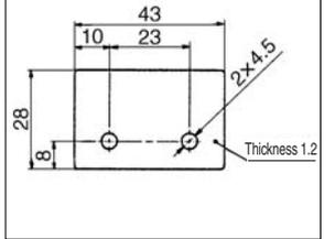
Spacer A is used to leave space for maintenance (for replacement of filter element etc.) on side mounting.
