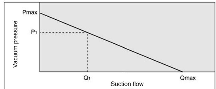
Flow characteristics are expressed in ejector vacuum pressure and suction flow. If suction flow rate changes, the vacuum pressure will also be changed. Normally this relationship is expressed in ejector standard use. In graph, Pmax is max. vacuum pressure and Qmax is maximum suction flow. The values are specified according to catalog use. Changes in vacuum pressure are expressed in the below order.
