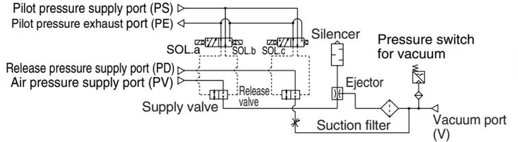
**With Function Plate/Applicable to Ejector System Only**
