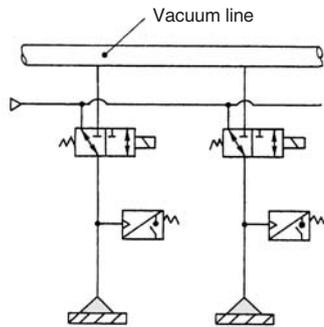
When pads and switches are common to one vacuum source, sometimes there is a possibility, depending on the number of adsorption and non-adsorption applications at each point in time, that the switches will not work within the range of set pressures due to pressure variations from the vacuum source. In particular, when small diameter nozzles are used for adsorption, the switches are greatly influenced by pressure variations. In order to remedy this situation, the following circuit is recommended.
