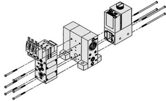
**Mounting Thread Parts List for Unit Combination**
