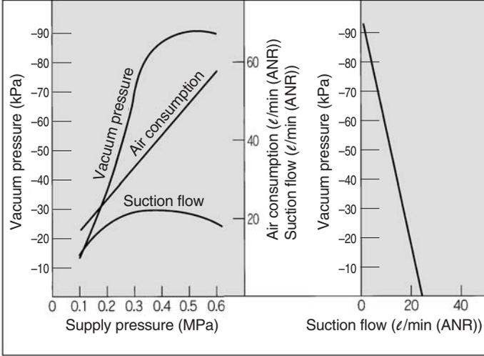
**ZR1-W18S1 Exhaust characteristics**      **Flow characteristics**
