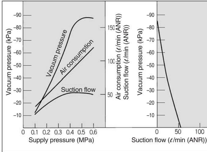
**Ejector Unit/Large Flow Type (L): Max. Vacuum Pressure -53 kPa**
