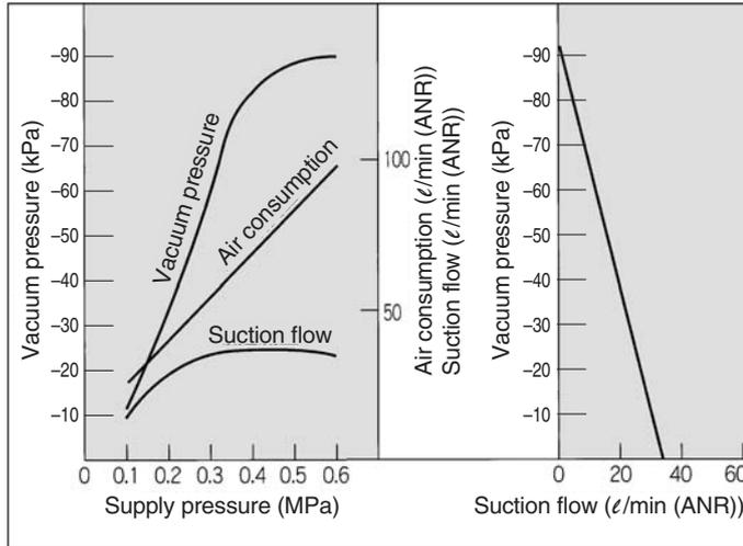
**ZR1-W20S1 Exhaust characteristics**      **Flow characteristics**
