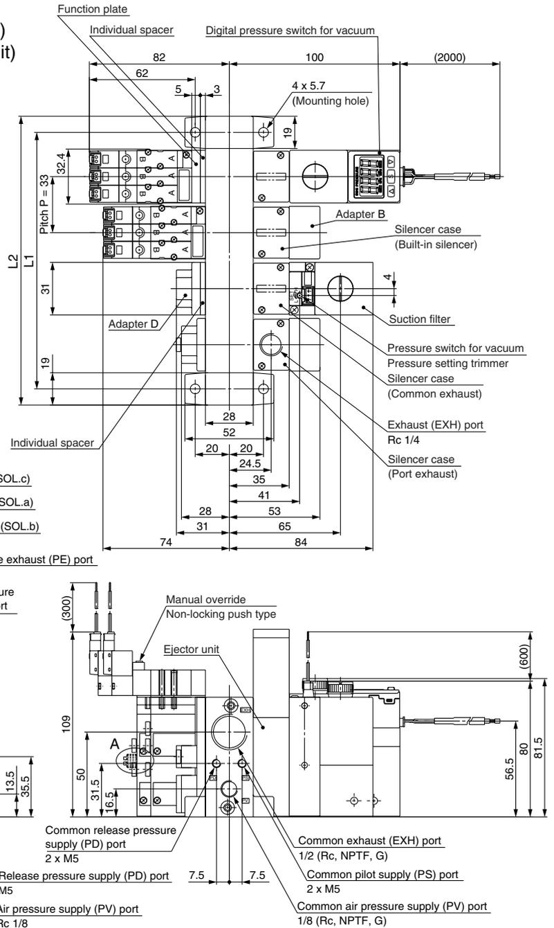
\* 1 The common exhaust port (EXH.) is also used as the pilot pressure exhaust (PE) port of the pilot valve. Use while the port is open to the atmosphere.
