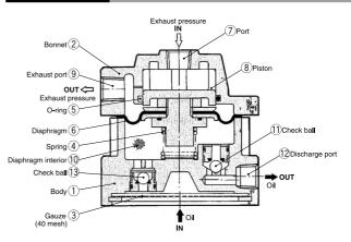
When the exhaust pressure from the switching valve enters into port  $\bigcirc$ , the piston  $\circledast$  and diaphragm  $\circledast$  compress and displace spring  $\bigcirc$ , the exhaust pressure is released into the atmosphere from exhaust port  $\bigcirc$ , and at the same time the diaphragm is relumed to its original condition by the recovery power of the spring.
