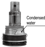
Grease deteriorates or is washed away.
