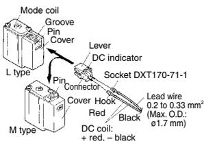
**Crimping lead wire and socket**
