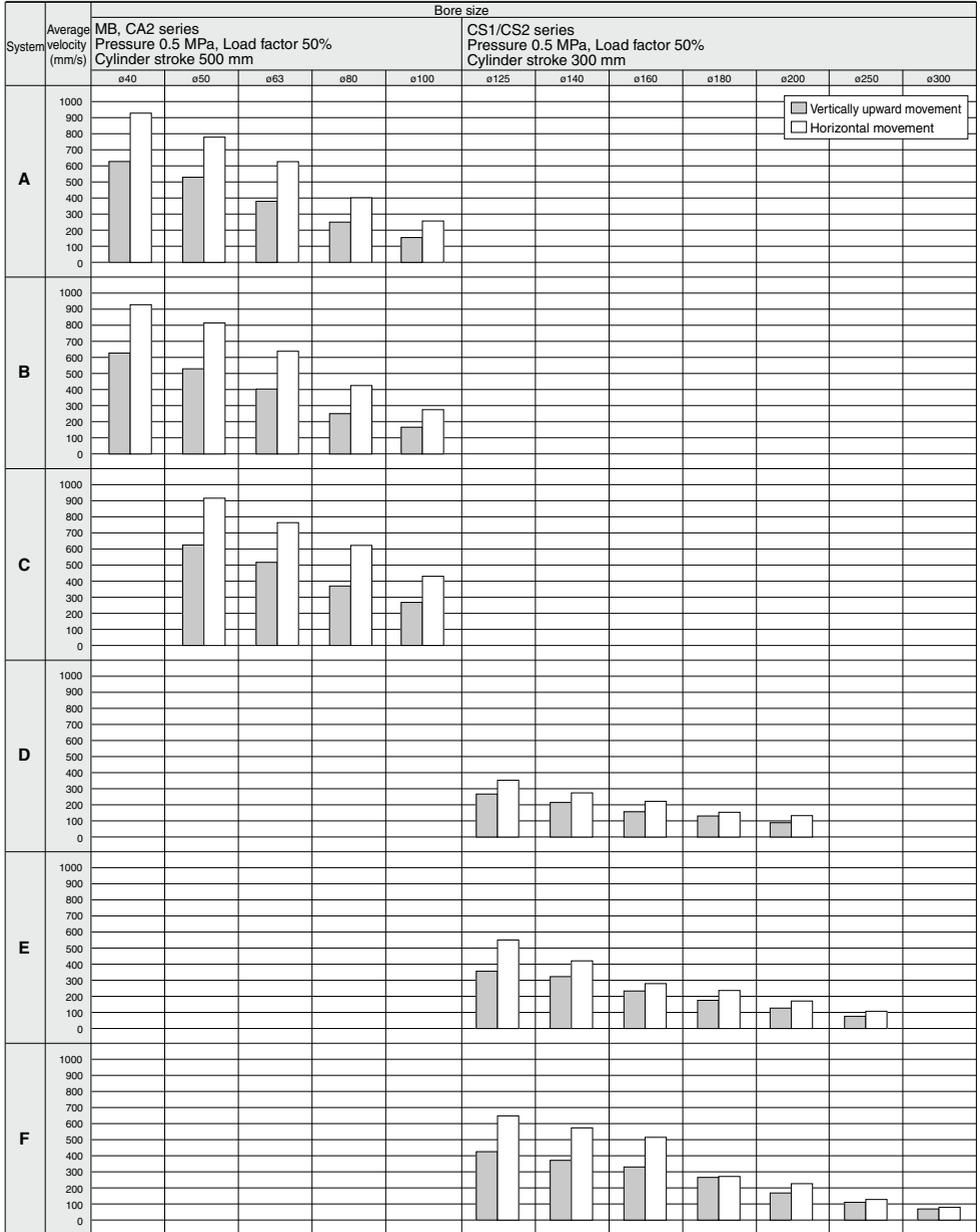
\* When the cylinder is extended, the speed controller is metered-out, is connected with the cylinder directly, and its needle is fully open.
