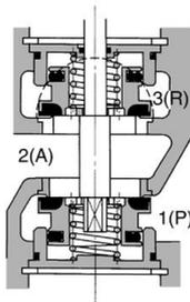
**(3) When Port 2 (A) pressure is low Pressure reducing supply**
