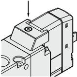
Push down on the manual override button with a small screwdriver until it stops. Release the screwdriver and the manual override will return.
