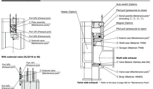
With solenoid valve (XLGV50 to 80)
