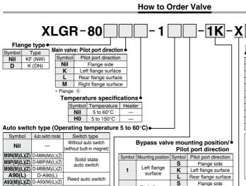
M9// Without auto switch (with built-in magnet) Note) Types with auto switches are not available in case of high temperature types. Standard lead wire length is 0.5 m. Add "L" to the end of the part number when 3 m is
