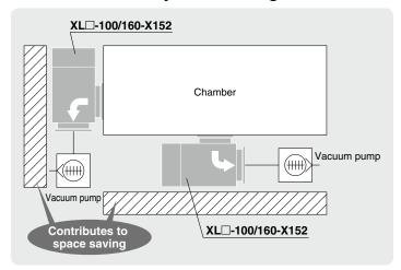
With restriction on exhaust direction (one way only: from valve element side to bellows side)
