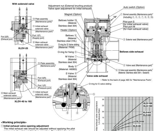
The initial exhaust rate should be adjusted without applying the pilot pressure to the pilot port S before operation. The initial exhaust rate is set to zero by gently turning the adjustment nut clockwise until it stops. (Do not use any tools.) The initial exhaust rate is adjusted by turning the adjustment nut counterclockwise.
