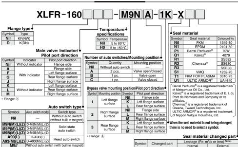
Note 1) Standard lead wire length is 0.5 m. Add "L" to the end of the part number when 3 m is desired, "M" when 1 m, and "Z" when 5 m.
