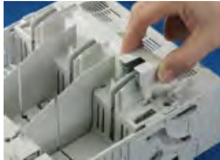
2. Clip the arc chambers into position
