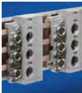
Bus-mounting fuse bases Screw-fastening or snap-mounting, 3-pole, for D02-E18, DII-E27 and DIII-E33 fuse technology.
