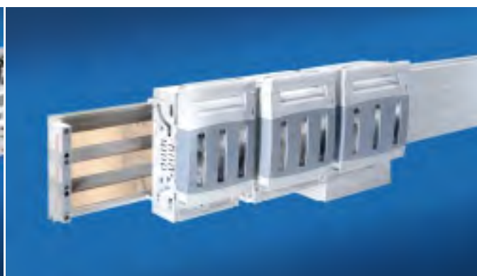
Fuse holder 100 to 400 A for mounting plate or busbar assembly 100 A/200 A/400 A fuse holders are intended solely for the use of J-Class fuses.
