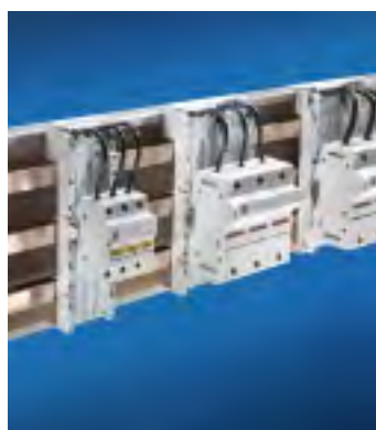
Fuse holder up to 60 A Simple mounting on support rails or via RiLine60 OM component adaptors on busbars.
