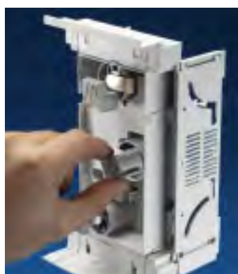
NH fuse-switch-disconnectors Size 00 to 3. Free choice of cable outlet (top/bottom) by simply rotating the mounting feet.
