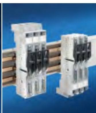
NH slimline fuse-switch-disconnectors Size 00. Free choice of cable outlet (top/bottom) by simply rotating the mounting feet.
