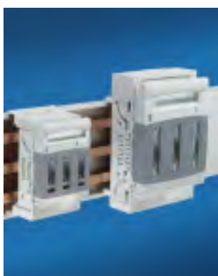
NH fuse-switch-disconnectors Size 00 to 3. Free choice of cable outlet (top/bottom) by simply rotating the mounting feet.
