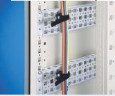
Velcro cable straps make cable management even easier because access to cables is unlimited and cables can be added or removed at will. The straps can be attached to cable collecting rails, C-rails, system rails or the enclosure frame. They can also be screwed to the standard installation holes in the enclosure frame with SZ 2486000 BZ 5.5 x 13mm screws (packs of 300).
