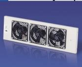
For 600 and 800mm wide TS cabinets. Designed for applications that require forced air cooling, mounts in side of enclosures frame or on system bars anywhere in enclosure. Can be used with either a perforated roof, a raised roof or 2 SK 3323207 exhaust filters.
