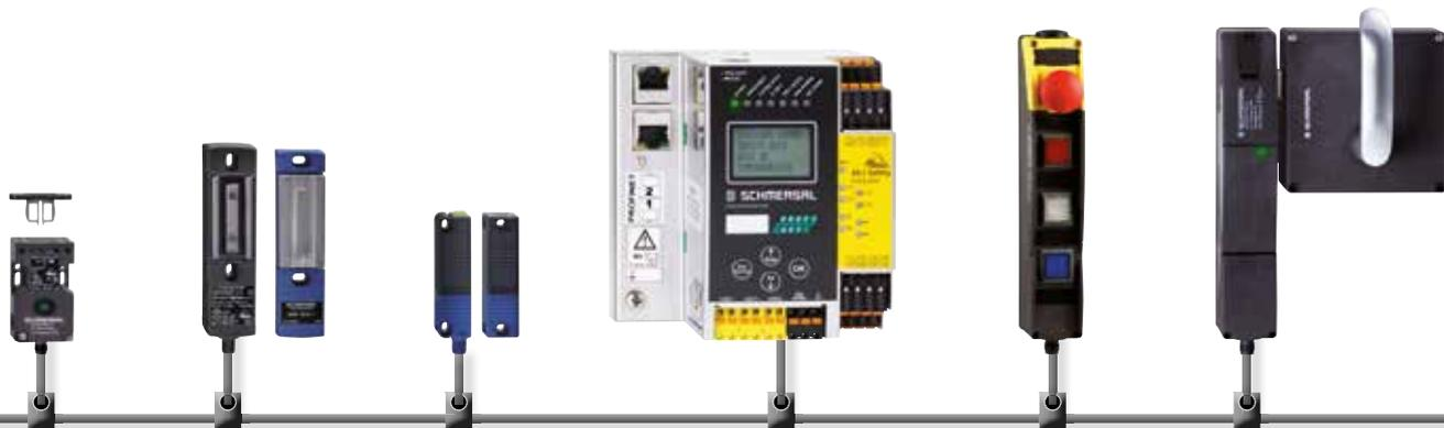
AS-Interface Safety at Work (AS-i Safety) is a safe bus system designed in accordance with the open AS International standard. Safety components such as emergency-Stop buttons, safety switches, solenoid interlocks and safety light curtains are connected via the unshielded 2-wire line of the AS interface which also supplies the components with energy.
