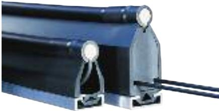
SCHMERSAL's rugged high-tear resistant rubber safety edges are available as sub-components or produced to user specifications. With a choice of aluminum mounting rails, they offer easy installation wherever crushing or shearing points must be safeguarded.
