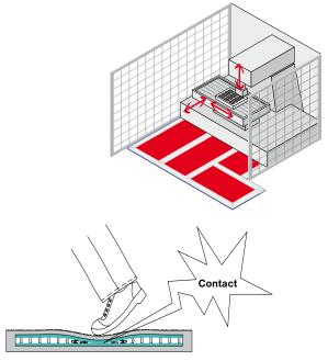
The safety mat consists of two separate current-carrying steel plates. The plates are held apart by insulating strips. Upon actuation of the pressure-sensitive safety mat, an electrical cross-wire short is produced between the steel plates. The connected safety-monitoring module evaluates this signal and stops the hazardous movement.
