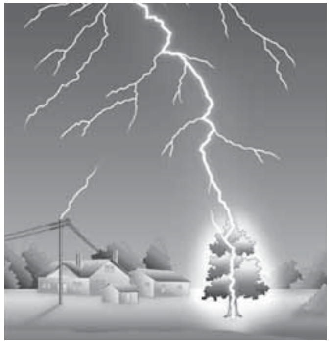
Figure 5. Upward leaders propagate toward downward leader to complete the ionized path between cloud and ground.
