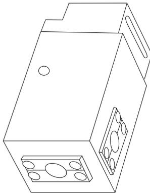
Wear Plates reduce mechanical abrasion of molds at cable entry points and help prevent leakage of molten metal (particularly on larger 7 strand conductor). These features prolong mold life.
