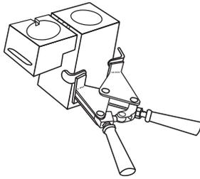
A semi-permanent graphite mold is used for making most CADWELD Connections. The mold controls the direction and speed of the molten CADWELD welding material flow and its final solidified shape. The graphite used in a CADWELD mold is a high temperature type that lasts for an average of 50 or more CADWELD connections under normal usage.
