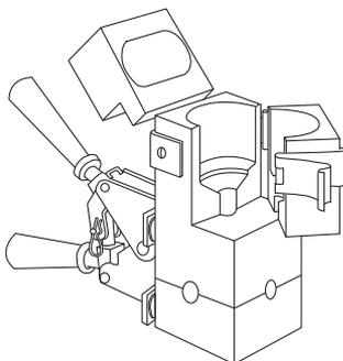
Molds made with a horizontal opening and solid crucible section may be specified as a SPLIT CRUCIBLE TYPE. The SPLIT CRUCIBLE MOLD allows for easier cleaning, but lead times are longer.
