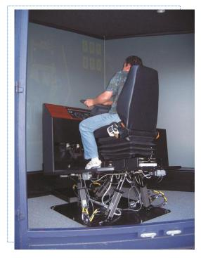
**Exlar Solution:** Six Exlar GSM20 actuators are used in the ThoroughTec mining equipment simulators. Two other families of linear actuators, the GSX Series and FT Series actuators are also available and offer varying stroke lengths, speeds, forces, and other mechanical characteristics to meet your application requirements.
