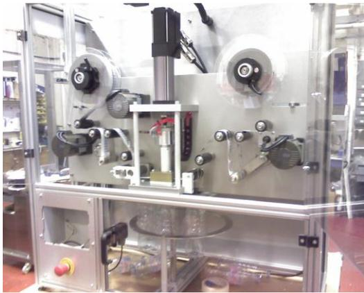
Cycle rates were increased using the high speed capability of Exlar's linear actuators - speeds as high as 40 linear inches/second, and with the control benefits of servo technology. This flexibility allowed Relco to adjust position and speed without setting any switches or changing offsets. They simply entered a new setting in the operator interface panel.
