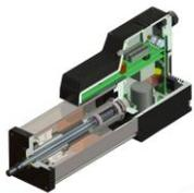
The roller screw is extremely efficient, provides very precise positioning capabilities and life counts in the hundreds of millions of cycles. The design allows the motor to be wrapped directly onto the outer shell; rotating the roller screw up to the full RPM's of the motor. This allows the linear movement to be as fast as 30 inches per second; perfect for high stroke needs on plunger pumps and sampling systems.
