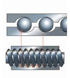
The depiction above illustrates the limited number of contact points in a ball screw compared to the contact points in a planetary roller screw design.
