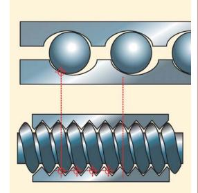
The greater number of contact points in a roller screw compared to a ball screw (above) gives roller screws a longer life, higher load capacity and greater stiffness.
