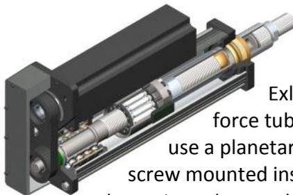
Exlar's FT Series force tube actuators use a planetary roller screw mounted inside a telescoping tube mechanism. An external motor supplied by Exlar or the customer provides the rotational force. FT Series actuators offer up to 8 foot stroke length and 40,000 lb force.
