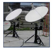
**Big** plans are in M<sup>2</sup>'s future with the help of the SmartMotor, including a cost-effective means of "auto-tracking." Auto-tracking is accomplished by writing code into the controller unit specifying a certain object's trajectory, while a separate antenna module with receiver is set up to judge signal strength of the object in orbit and automatically adjust the equations in the system to correct the slightest position error and therefore receive the strongest signal data.
